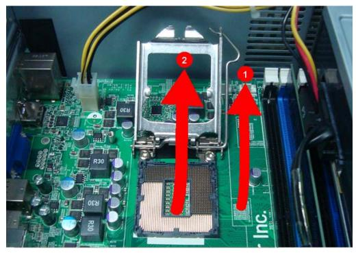
3. Gently put the processor to the socket., then close the retention plate and the load lever to its latch.
